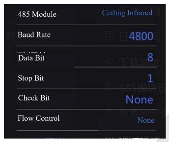
② 485 Protocol control: Enabling operations such as play, stop and switching of clips via third-party commands (for details, please refer to the control protocol).
