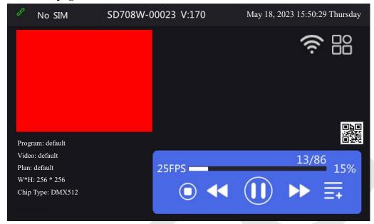
The top of the interface features the display of the network signals, controller ID number as well as the date, time and version of the device software.
